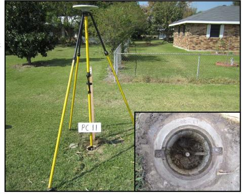
\* The surveyed information referenced above is the mean of multiple static GPS observations uploaded to NGS for OPUS processing utilizing the Geoid09 model.
